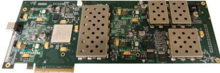
**Figure 2: Quantum Random Number Generator PCIe card.**
